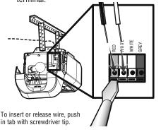
**PRE-WIRED INSTALLATIONS:** Connect the same wires to the garage door opener that were previously connected to the door control.
