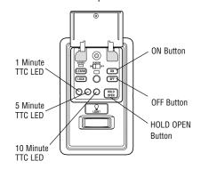
**NOTE:** If you have an 880LM installed and the TTC is set to a custom time, the 3 LED's on the 881LM will blink. If the 3 LED's are blinking and you have an 881LM ONLY, press the ON button to set the time properly.
