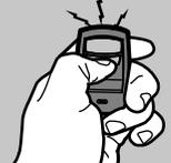
**4** To exit programming mode, press any remote control button **except** the button that was just programmed.
